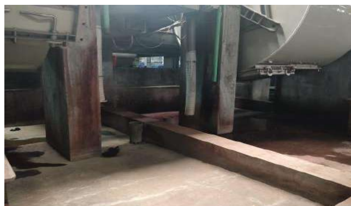
Picture 3: One of the tanneries visited connected flexible pipes from drums to segregate discharge
